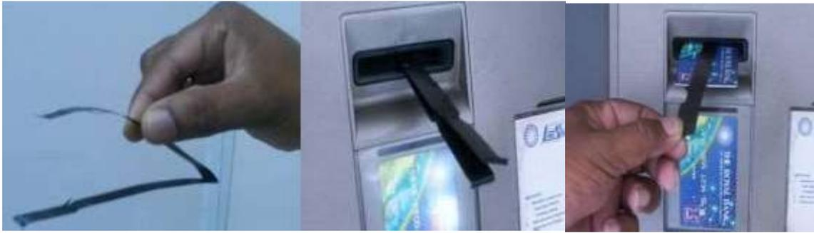
**The Lebanese loop** is a device for blocking the card reader, it is made as a loop from an old film, designed to steal bank cards.
