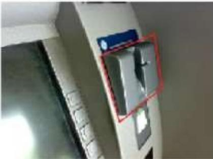
**Skimmer** is an overlay inside which there is a device that reads information from the magnetic strip of the payment card. In the future, this information will be used to make a duplicate card. Typically, skimmers are attached to the ATM to find out the PIN code, scammers use hidden video cameras and overhead keyboards.
