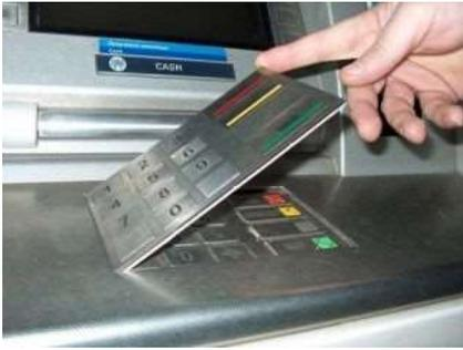
**The EPP keyboard cover** is a skimming device made in the form of an EPP keypad designed to copy the PIN code of a bank card.
