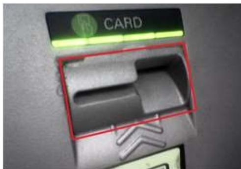
**The overlay on the card reader** is a skimming device made in the form of a card reader, intended for copying data from a chip or a magnetic strip of a card.
