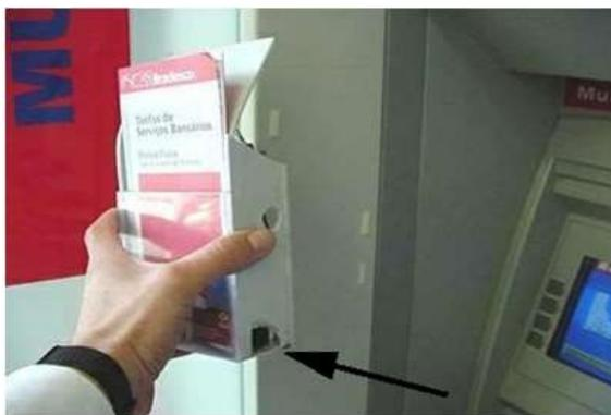
**Video Camera** - concealed device manufactured in the form of various bank supplies: parts ATM (card reader, cash dispenser lining on walls, wall paper holders, etc.). It is designed to record a PIN code of a bank card.
